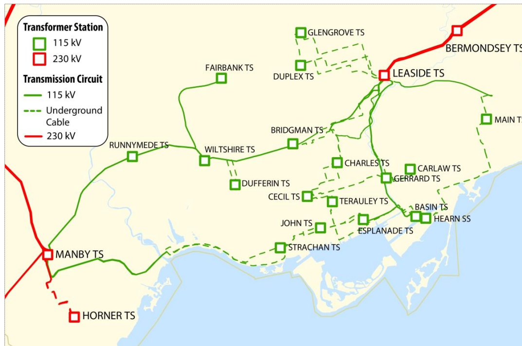
Figure 1-2 Electrical Supply in Central Toronto (Inset)
