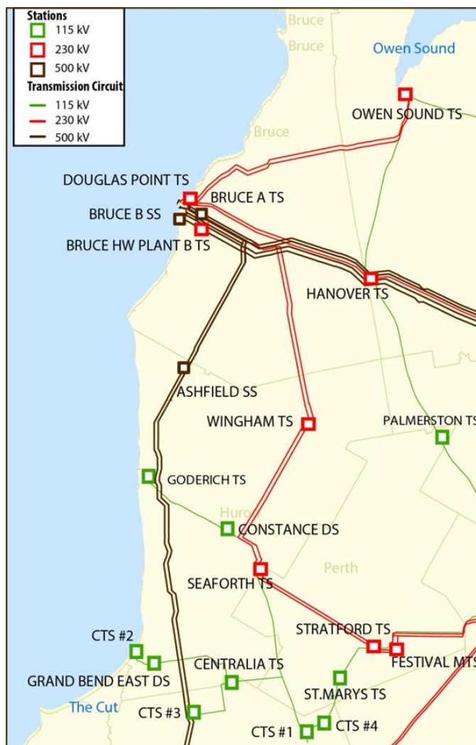
Figure 1: Electricity Infrastructure in the Greater Bruce/Huron Region 2
