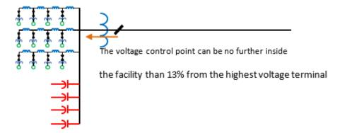
**Figure 14 - Voltage Control Point**
