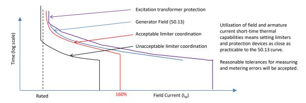
Figure 18 - Temporary Field Current Requirements
