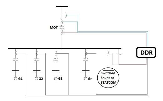
**Figure 2 - Dynamic Disturbance Recorder Inputs**
