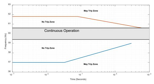
Figure 3 - Off-Nominal Frequency No-Trip Requirement
