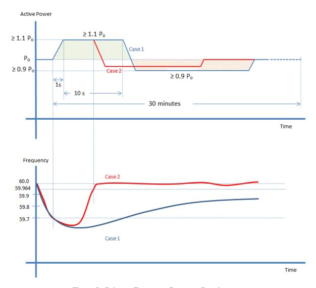
Figure 5 - Primary Frequency Response Requirement
