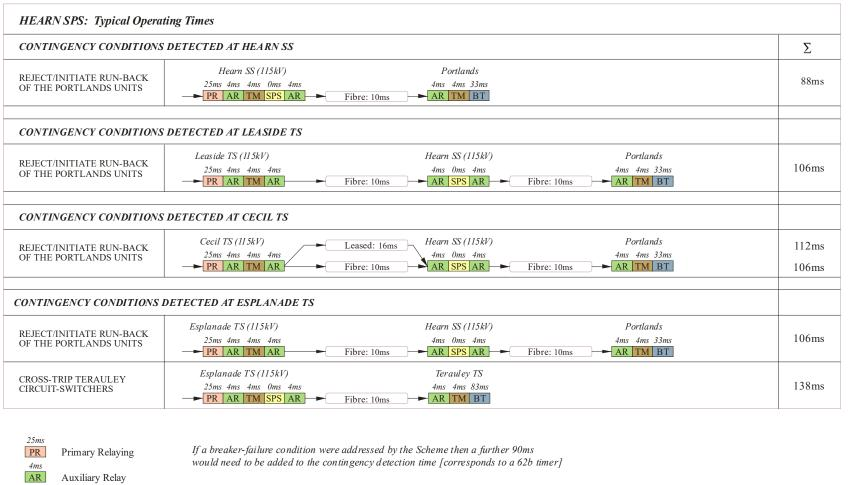
Trip Module SPS Matrix 33ms (For a 2-cycle breaker) Breaker Trip Time
