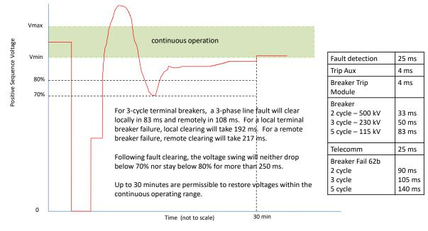
Figure 9 - Positive Sequence Voltage During a Fault
