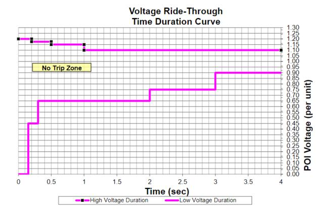
Figure 6 – NERC PRC-024 Voltage Ride Through Requirement
