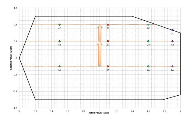
Figure 13 - Regulation with Individual Units at Limit
