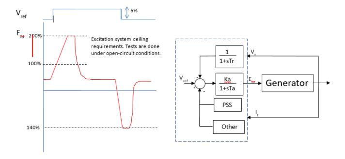
**Figure 16 - Excitation System Ceiling Requirements**
