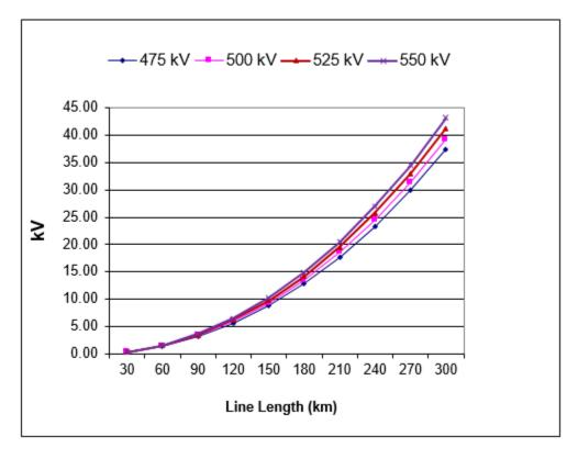
Figure 2: 500 kV LEO Voltages
