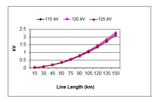
Figure 4: 115 kV LEO Voltages
