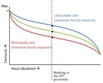
The forecast in the 3<sup>rd</sup> percentile was considered the "Extreme Peak" (extreme profile, red curve) and the forecast in the 50<sup>th</sup> percentile was chosen was the "Median Peak" (median profile, green curve). For the Niagara IRRP, the median profiles were scaled to their respective maximums from the peak demand forecast.
