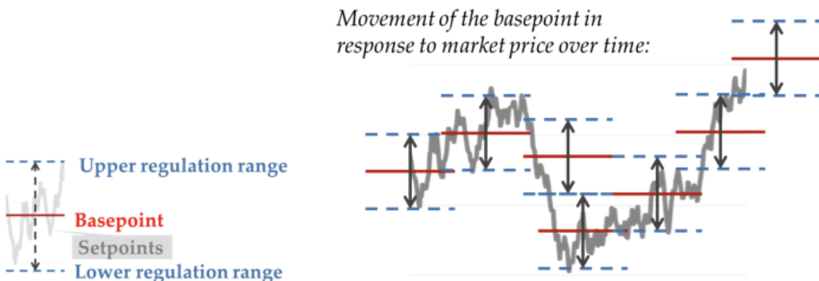
Figure 2-14 - Illustration of the setpoint and basepoint movements of a standard regulation signal for a generation facility
