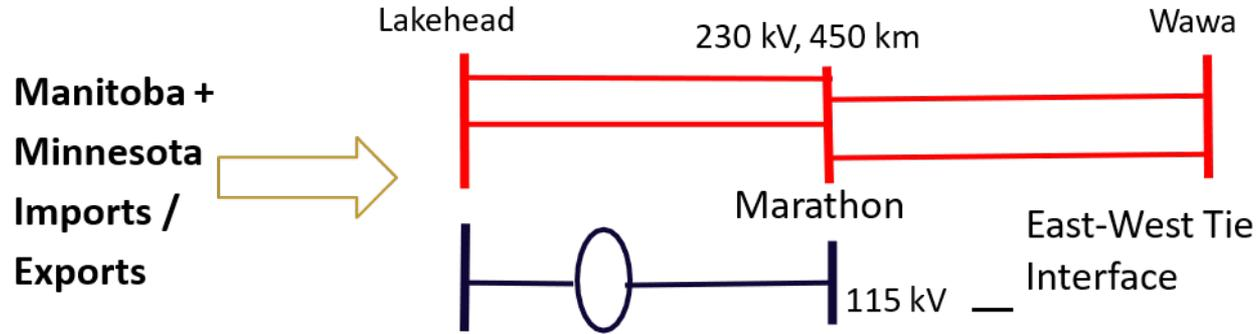
The EWT Expansion project consists of a new, double-circuit 230 kV line which parallels the existing EWT line from Lakehead TS to Wawa TS (with switching at Marathon TS).
