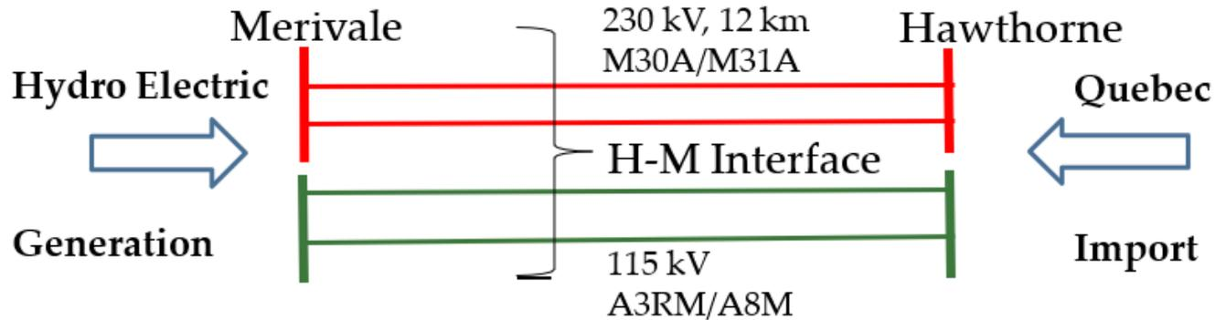
The Hawthorne to Merivale 230 kV Upgrade project consists of reinforcing the existing M30A/M31A circuits between Hawthorne TS and Merivale TS in the Ottawa area
