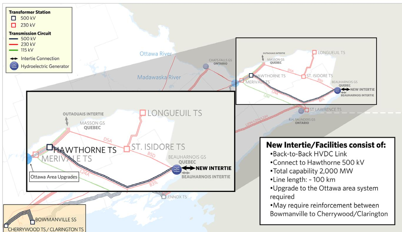
The new interconnection comprises a conventional HVDC bipole line rated 500 kV and 2,000 MW with the rectifier terminal at Quebec’s Beauharnois station and the inverter at Ontario’s Hawthorne 500 kV switchyard. Another feasible configuration is, instead of a conventional HVDC bipole line, a back-to-back DC link located at Quebec’s Beauharnois station and from there, a double-circuit 500 kV AC line from Beauharnois to Hawthorne would be constructed.
