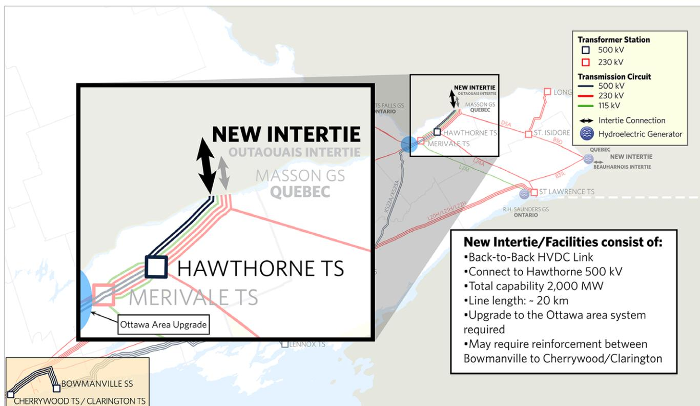
The new interconnection comprises an additional back-to-back DC terminal rated 2,000 MW at the Outaouais station in Quebec. From there, a double-circuit 500 kV transmission line (or underground cables) connects the new DC Link at Outaouais to the 500 kV switchyard at Hawthorne TS. A variation of the above is, instead of a back-to-back DC link, the Outaouais to Hawthorne connection would be a conventional HVDC bipole line rated 500 kV and 2,000 MW.
