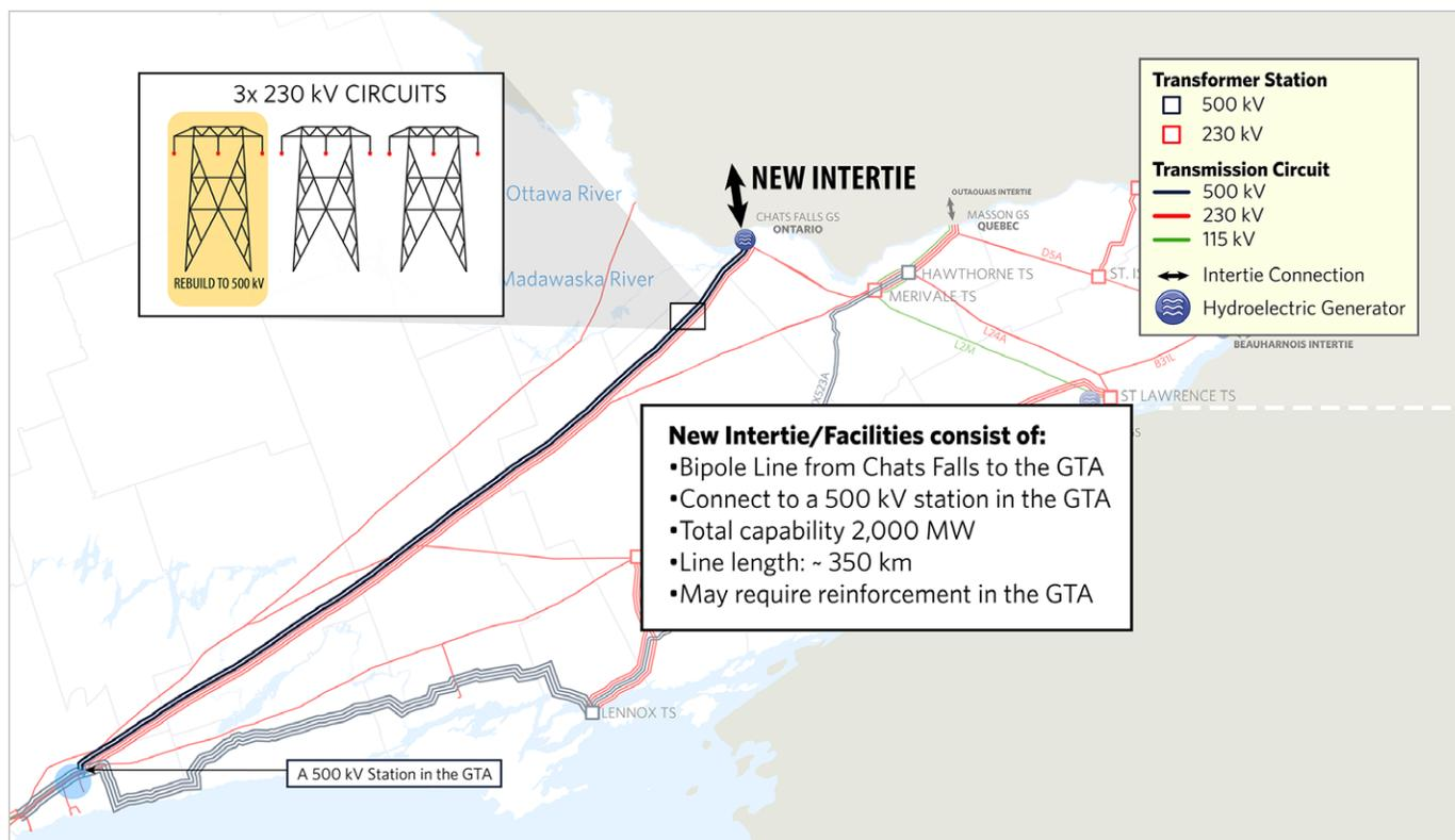
The new interconnection comprises a conventional HVDC bipole line rated 500 kV and 2,000 MW with the rectifier terminal at a new Quebec's station near Chats Falls and the inverter at a major station in the GTA. An alternative to that is to construct two 1,000 MW 230 kV bipole HVDC lines. Most likely, the HVDC line(s) would utilize the existing 230 kV "Gatineau" corridor from Chats Falls to the east GTA.
