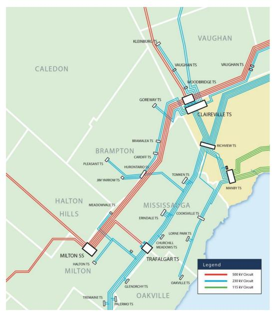
**Figure 1 Geographical Area of the GTA West Region with Electrical Layout** Source: IESO
