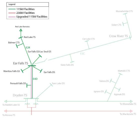
Figure 29: New 115 kV line to Ear Falls Diagram
