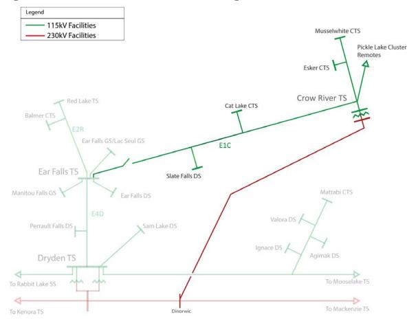
Figure 33: New 230 kV line to Pickle Lake Diagram
