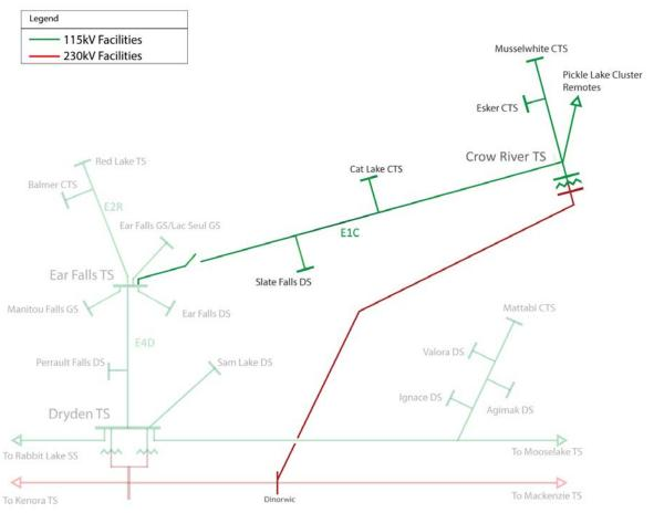
Figure 21: 230 kV Line Option Pickle Lake Subsystem Configuration
