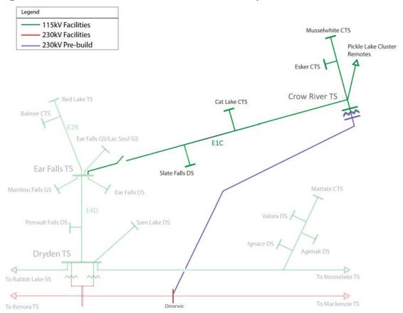
Figure 35: Pre-build 230 kV Line to Pickle Lake Option
