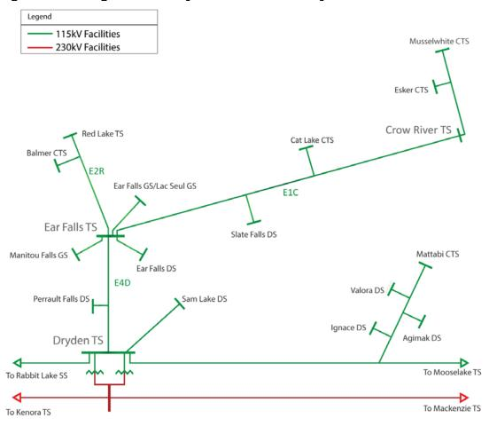
Figure 6 Existing North of Dryden Transmission System
