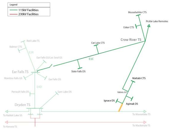
Figure 31: New 115 kV line to Pickle Lake Diagram
