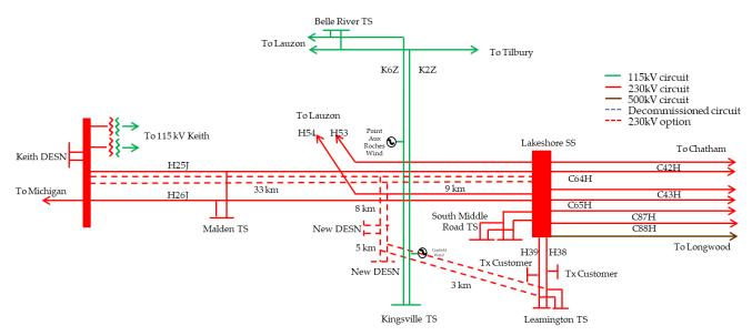
Figure 16 | Potential Long-Term 230 kV Reinforcement Between Keith and Lakeshore
