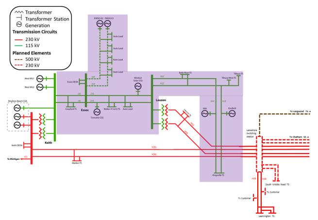
Reliability in this sub-system is thermally limited by the 115 kV circuits between Keith and Essex, J3E and J4E. This phenomenon depends on assumptions for the load level of the 115 kV network, the output of generation facilities in Windsor, and imports/exports at J5D, but is particularly relevant for three contingencies:
