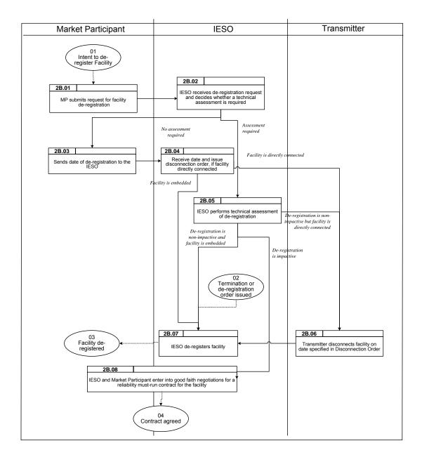
Figure 4-1: Workflow for Facilities De-registration
