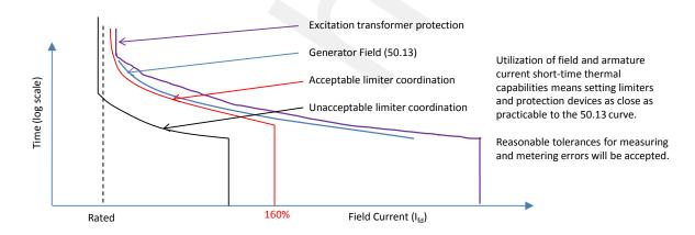
**Figure 17 - Temporary Field Current Requirements**
