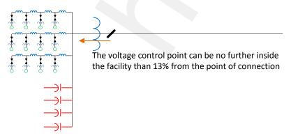
**Figure 13 - Voltage Control Point**
