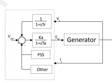
**Figure 15 - Excitation System Ceiling Requirements**
