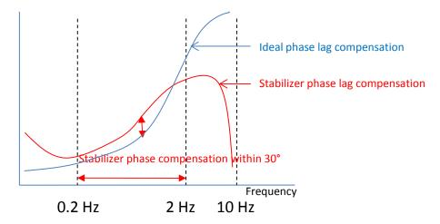
Figure 16 - Power System Stabilizer Phase Compensation Margin
