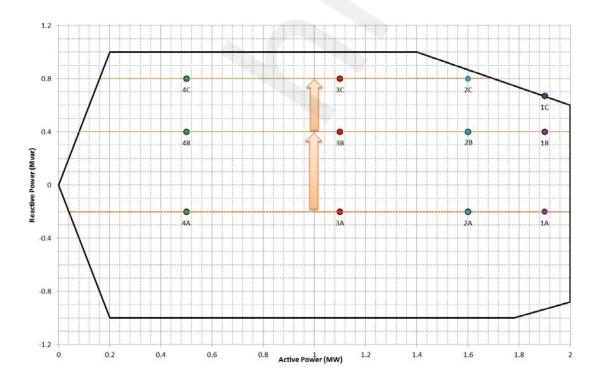
Figure 12 – Regulation with Individual Units at Limit
