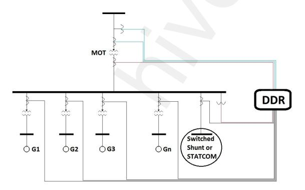
Figure 2 – Dynamic Disturbance Recorder Inputs
