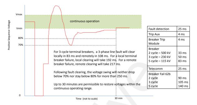
Figure 8 - Positive Sequence Voltage During a Fault
