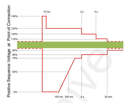
Figure 5 - Voltage Ride Through Requirement
