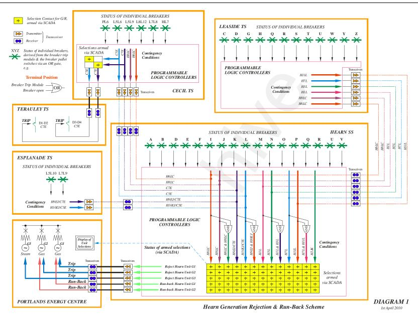
Figure 20 - Special Protection System Matrix
