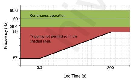
Figure 3 - Off-Nominal Frequency No-Trip Requirement
