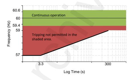
Figure 3 - Off-Nominal Frequency No-Trip Requirement
