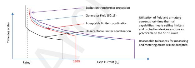
Figure 18 - Temporary Field Current Requirements
