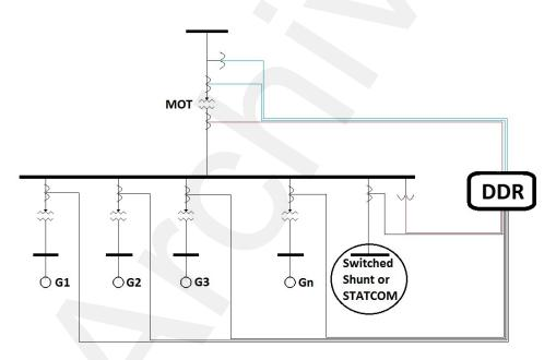
**Figure 2 – Dynamic Disturbance Recorder Inputs**
