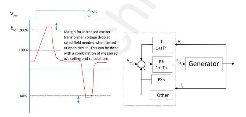
Figure 16 - Excitation System Ceiling Requirements
