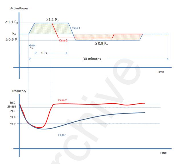
**Figure 5 – Primary Frequency Response Requirement**
