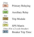
If a breaker-failure condition were addressed by the Scheme then a further 90ms would need to be added to the contingency detection time [corresponds to a 62b timer]
