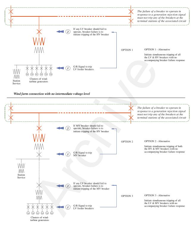
Wind farm connection with an intermediate voltage level
