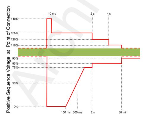
Figure 6 - Voltage Ride Through Requirement
