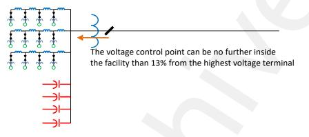
Figure 14 - Voltage Control Point
