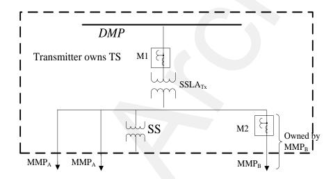
$MMP_A$  and  $MMP_B$  are directly connected to the TS bus inside the fence  $MMP_A$  and  $MMP_B$  are  $\it transmission \it customers$
