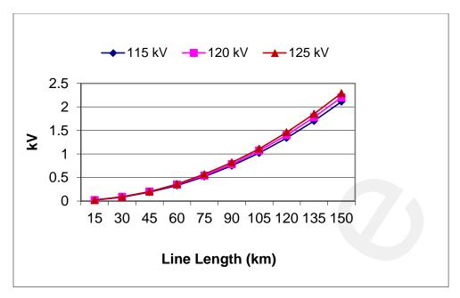
Figure 4: 115 kV LEO Voltages
