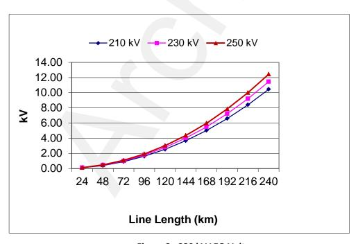
Figure 3: 230 kV LEO Voltages
