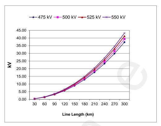
Figure 2: 500 kV LEO Voltages
