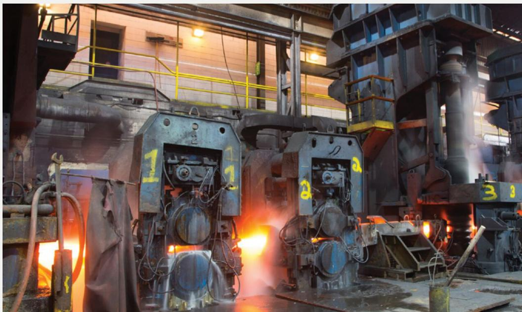
In the Gerdau Steel plant in Whitby, Ontario, temperatures in the arc and ladle furnaces that produce some of the world's greenest steel reach temperatures exceeding 1600 degrees Celsius. The significant energy required to melt 700,000 tonnes per year of scrap metal, and then roll it into recycled steel products such as rebar, is the main reason why Gerdau's energy team decided the time was right to participate in the IESO's Demand Response (DR) auction.
