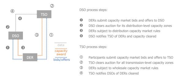
Figure 7: Illustrative coordination process for capacity procurement in Hybrid DSO Model
