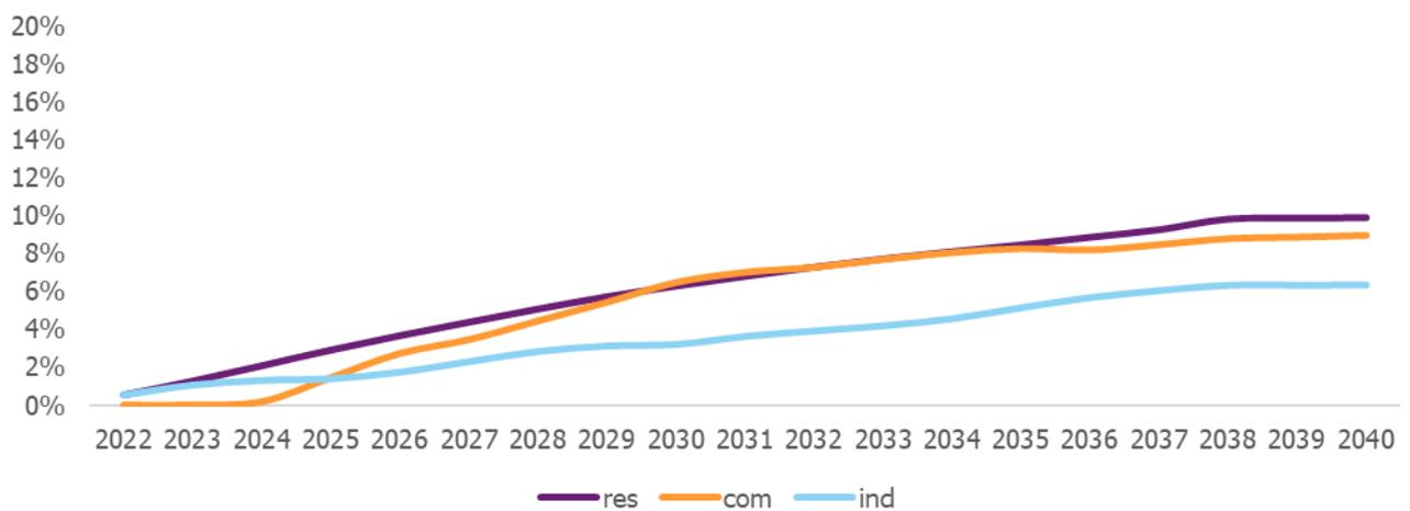
Applying these rates of uncommitted savings potential to the demand forecasts for Vineland DS, indicates that about 2 MW of CDM savings are available among customers connected to this station in 2041. The estimated cost to deliver these savings is \$6.4 million dollars over the forecast period based on APS cost assumptions.
