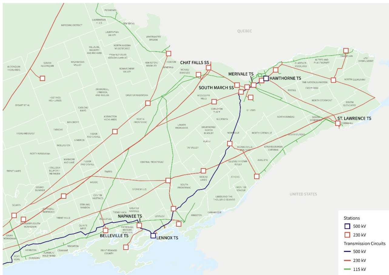
Figure 1 | Eastern Ontario Transmission Network
