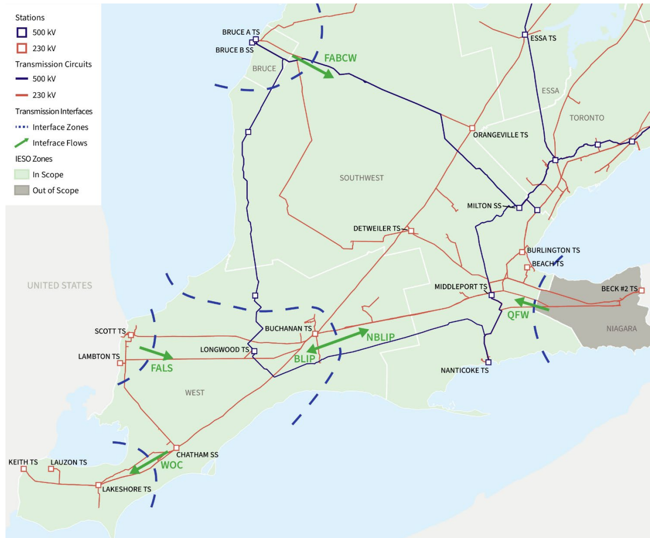
Figure 17 | Major Interfaces in Southwestern Ontario
