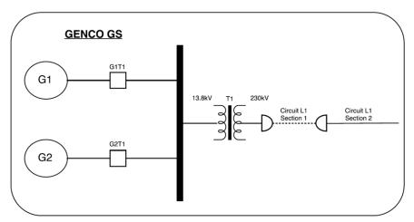
Figure 3-1: Single-Line Diagram Example
