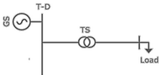
1a. Existing generating station (GS), transformer station (TS), load
