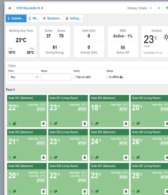
Real time optimisation of electric heating circuits to improve comfort and eliminate needless waste of energy
