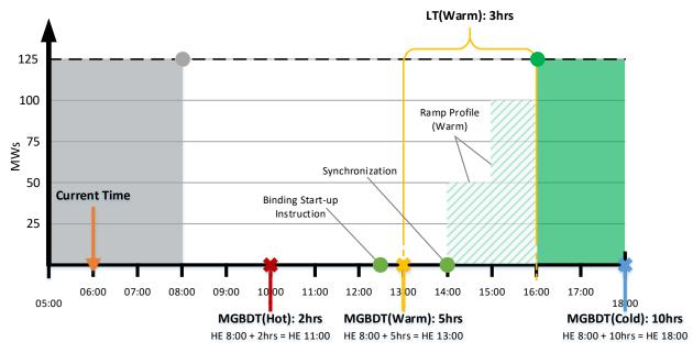
As illustrated in **Figure 7**, the PD scheduling process calculates that there are eight hours between when Generator A will end its commitment at 08:00 and when it will be needed again at 16:00. The scheduling process then determines that Generator A will be warm at 16:00 by comparing the length of the time it will have been below its MLP (i.e. eight hours) to its MGBDT data. Generator A enters a warm state after
