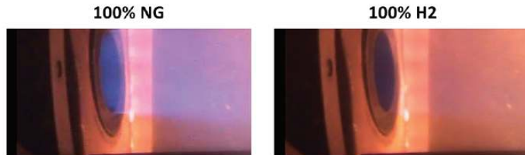
Figure 1: Comparison of hydrogen & natural gas flames, H2 flame is invisible (Source: GEA 33861)
