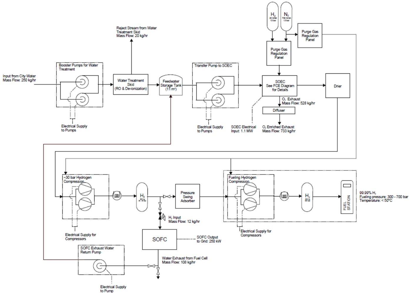
Water is the primary feedstock for the system and is fed at ambient conditions at a rate of 230 kg/hr. This water undergoes a purification process to reduce its conductivity to 1  $\mu\text{S}/\text{cm}$ , ensuring the production of deionised (DI) water. The DI water is stored in an 11 m<sup>3</sup> reservoir, from where it is supplied to the 1.1 MW SOEC unit at the ideal operational pressure of 2 bar.
