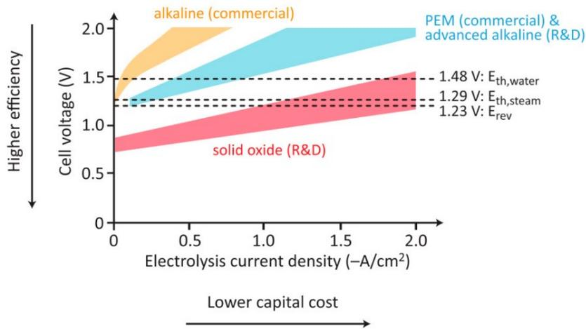
As temperature increases, the energy efficiency of SOECs improves. The integration of individual cell stacks, or multiple stacks makes SOECs very efficient. The system can recover and effectively use energy, resulting in an approximate overall system efficiency of 95%. However, it is important to note that high-temperature operation is a double-edged sword. Although efficiency is improved, stack failure is more likely or is accelerated due to thermal stress.
