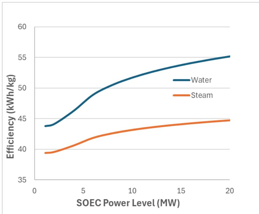
Figure 21 shows that as the power level increases, the efficiency tends to decrease (i.e. the energy consumption per kilogram of hydrogen produced increases). SOECs maintain competitive efficiency across this range, typically between 37.5-55 kWh/kg. This trend is consistent with the inherent thermal and electrical losses that scale with system size.
