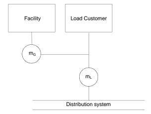
An In Series connection configuration is only permitted at the discretion of the LDC. Battery back-up and supply systems are not permitted for an In Series connected Facility.
