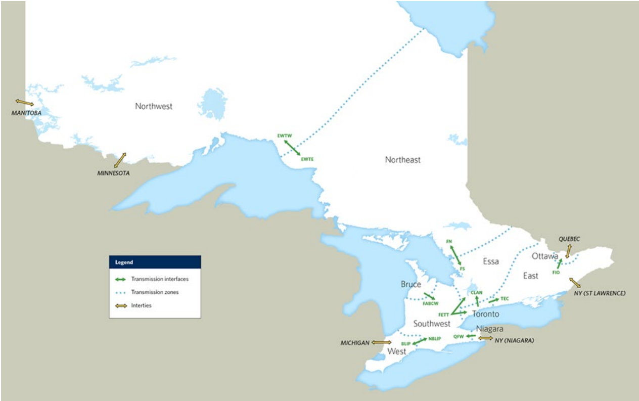
Figure 16 | Ontario’s Major Transmission Interfaces, Electrical Zones and Interties
