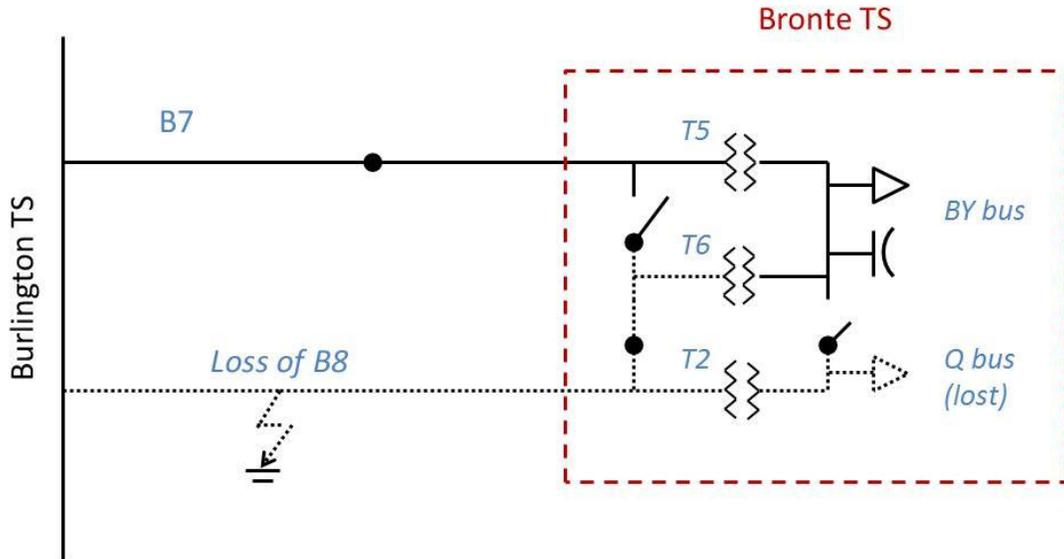
Following the loss of circuit B7, all Bronte TS load is served by the T2 and T6 transformers and sudden voltage drop becomes a constraining need. Note that this is the same contingency which was found to be more limiting when considering thermal limits of the supplying B7 and B8 circuits, as described in Section B.3.1.
