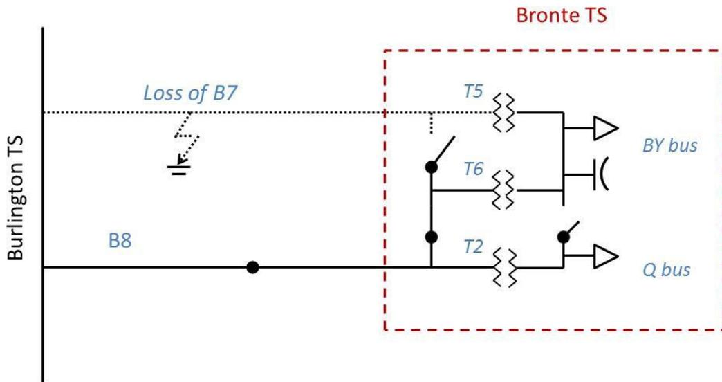
Under this contingency, the need is sensitive to the distribution of load between the two buses (BY and Q). This means that the maximum allowable station capacity varies depending on where the load is assigned. Of the two distribution side buses, BY is slightly more sensitive to sudden voltage drops. The graph below shows the loading conditions that produce a 10% voltage drop on the BY bus following the loss of B7:
