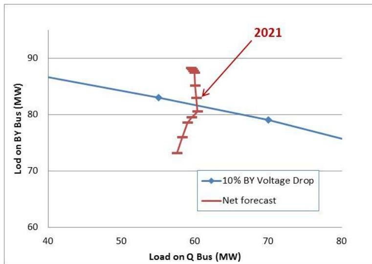
The area underneath the blue line represents “operable” loading profiles. This means combination of BY and Q bus loading which will not cause a voltage drop of over 10% on the
