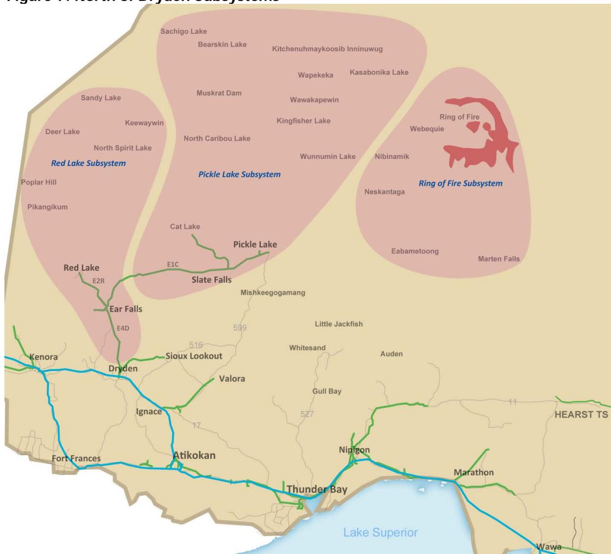
The Ring of Fire subsystem does not include any existing transmission facilities. The subsystem includes five remote communities that are identified for connection in the 2014 Remote Community Connection Plan as well as potential future industrial customers at the Ring of Fire mine development area.
