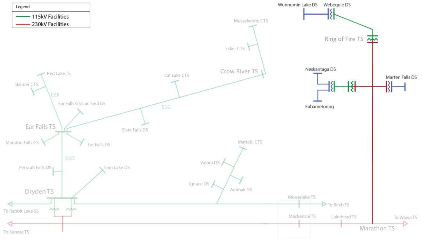
The LMC of the Ring of Fire subsystem for this option is 77 MW. This includes 7 MW for the communities on the line as well as 70 MW at the Ring of Fire. A summary of the cost for this option can be found in Table 102 below.
