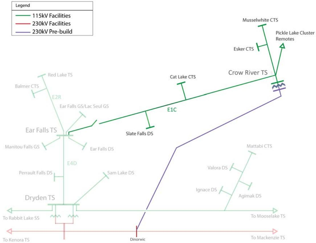
Note: the above diagram illustrates the second stage configuration (operated at 230 kV).
