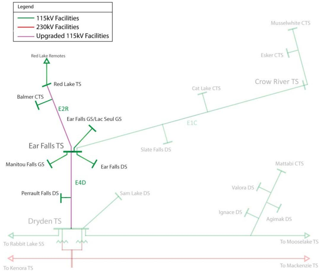
Figure 23: E4D and E2R Upgrade Red Lake Subsystem Configuration
