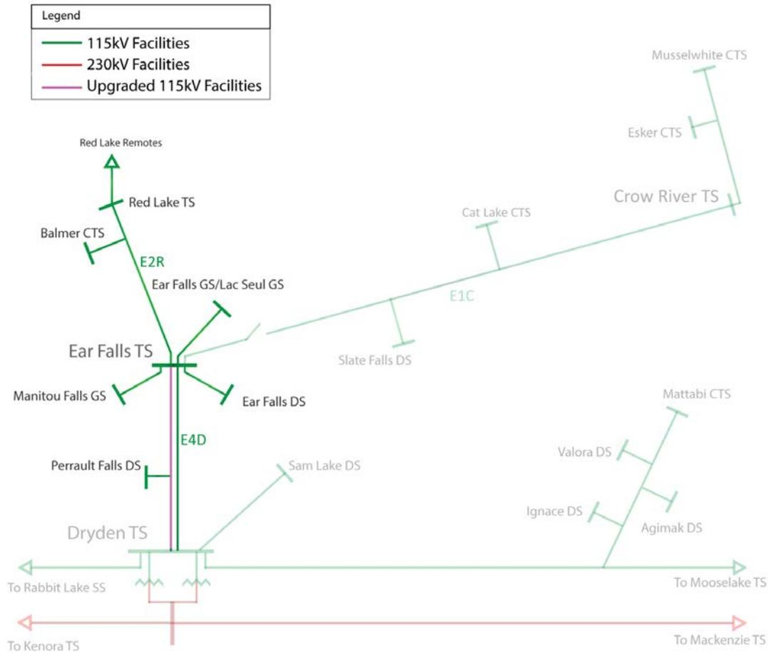
Figure 30, shows the peak load flow case for this option. Voltage at Ear Falls TS is maintained within a healthy range of 120 kV to 125 kV.
