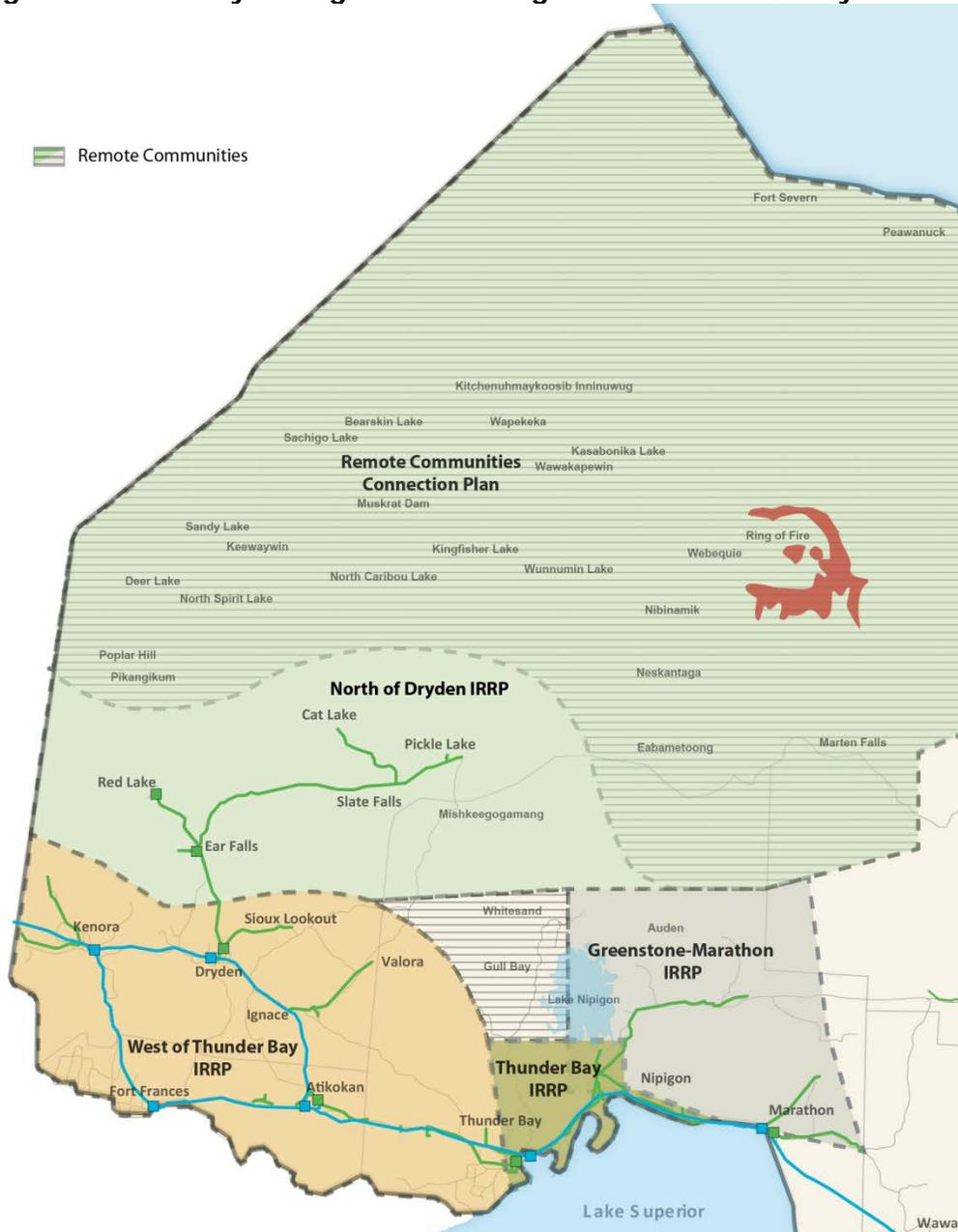
The transmission system supplying the North of Dryden sub-region is currently at capacity. This IRRP recommends options to provide new high voltage electrical capacity to meet near-term growth, while providing options to meet future growth as it becomes more certain. These near-term recommendations are presented as action items for immediate or early deployment. Options to address potential longer-term needs are also
