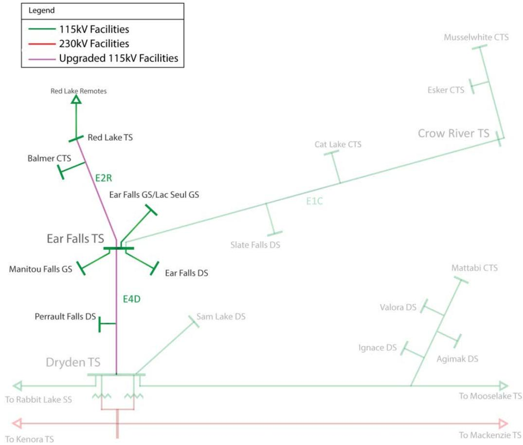
Hydro One has indicated that upgrading these lines as well as the installation of required voltage control devices could be completed within the near-term period. Table 86 below shows the cost breakdown of the upgrade option which includes the required voltage control devices. Figure 28 shows the load flow case during peak load. Ear Falls TS and Red Lake TS voltage is maintained in a healthy range of 120 kV to 125 kV.
