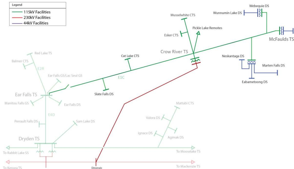
A prorated portion of the costs for new a 230 kV transmission line and 230/115 kV transformer station from the Dryden area to Pickle Lake is included in the cost of this option because it is required for this option to be undertaken as is shown in the cost summary in Table 99.
