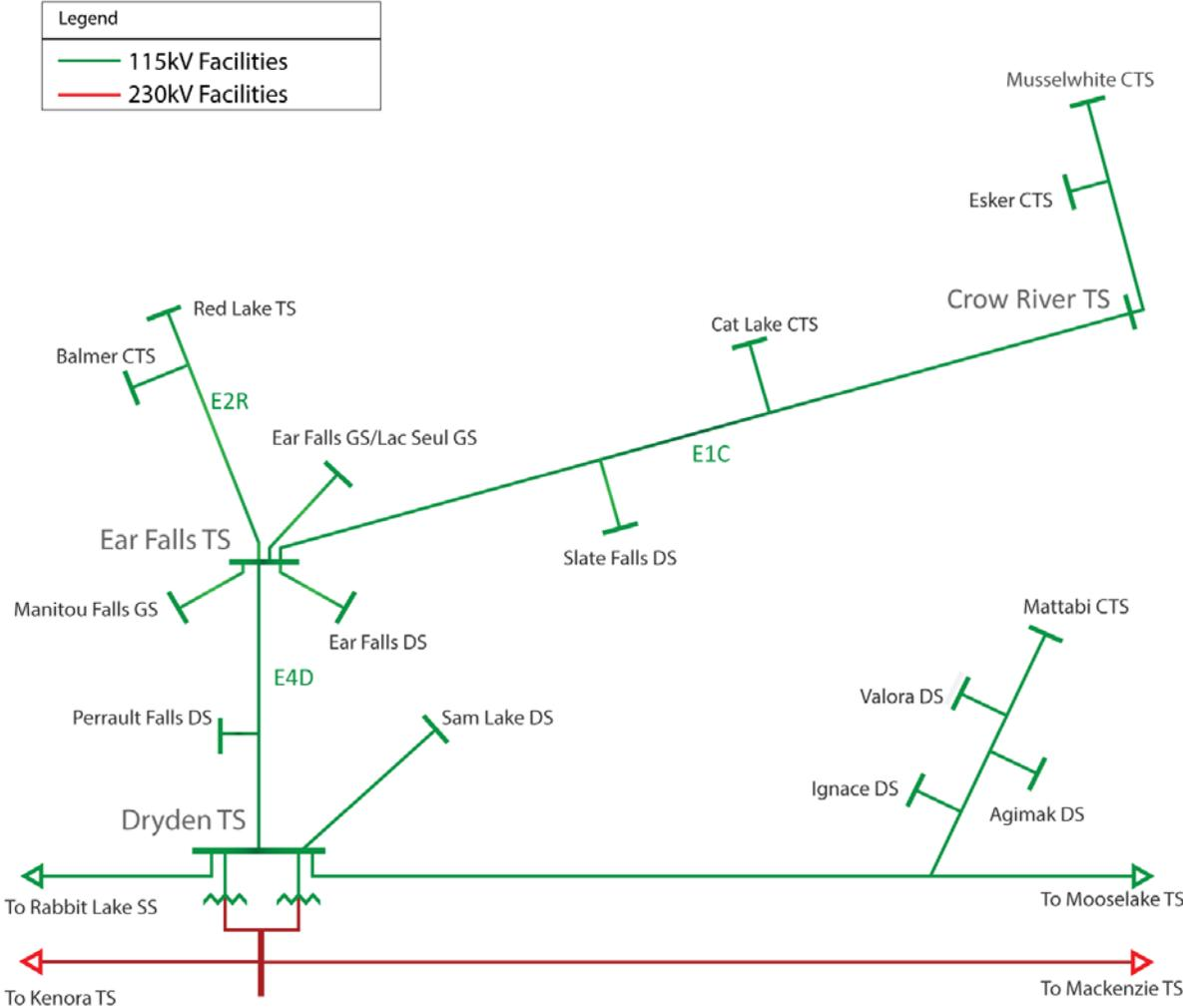
Figure 19: Existing North of Dryden Transmission System Load Flow Plot
