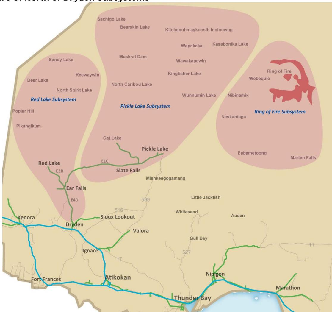
Where growth in electricity demand identified in these subsystems cannot be met by the existing system, technically feasible conservation, local generation, and transmission options are identified and compared based on their ability to cost effectively meet the needs.
