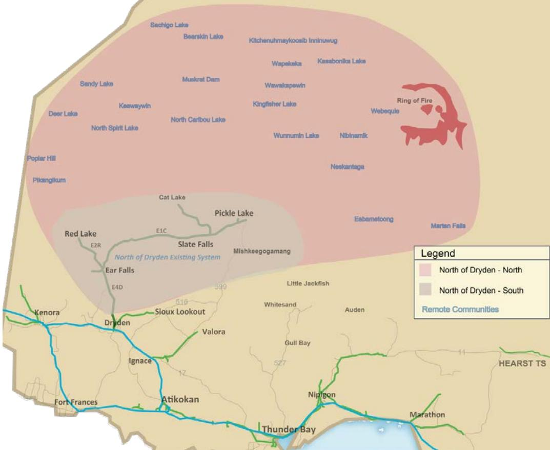
The North of Dryden sub-region is forecast to experience some of the highest growth in electrical demand in Ontario. Currently the electricity transmission system serving the area is at capacity and is unable to accommodate demand growth.
