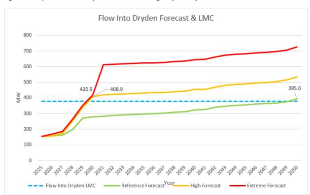
Figure 6.2 | Flow into Dryden Load Meeting Capability and Forecast Scenarios
