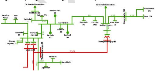
Figure 5-3 | Single Line Diagram of the Dryden Area
