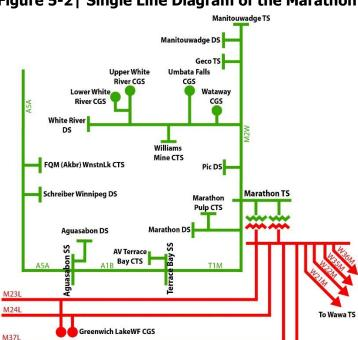
Figure 5-2 | Single Line Diagram of the Marathon Area
