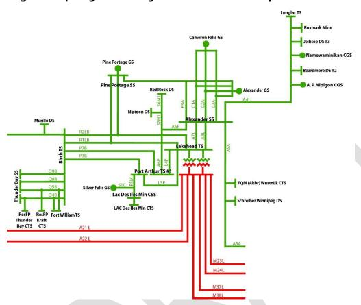
Figure 5-1 | Single Line Diagram of the Thunder Bay Area
