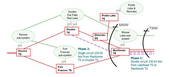
Based on the application of planning criteria to the existing system configuration, the interface being reinforced by Phase 2 has a higher transfer capability today than that of the interface being reinforced by Phase 1
