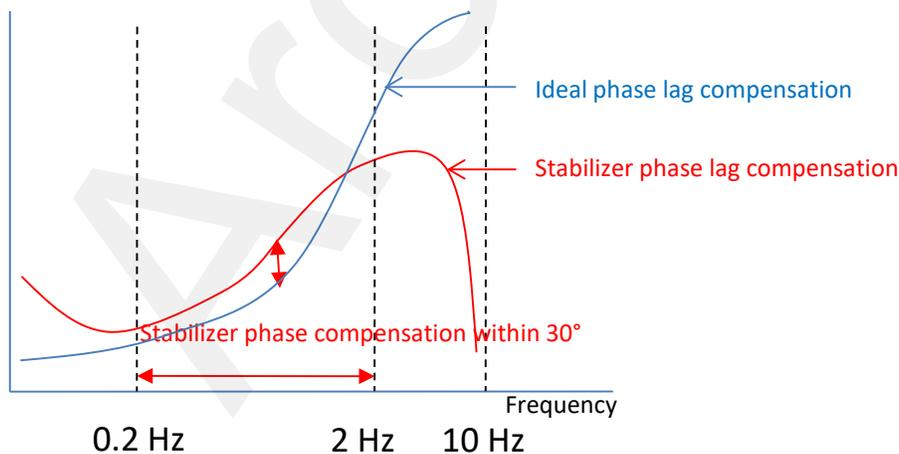
**Figure 17 - Power System Stabilizer Phase Compensation Margin**
