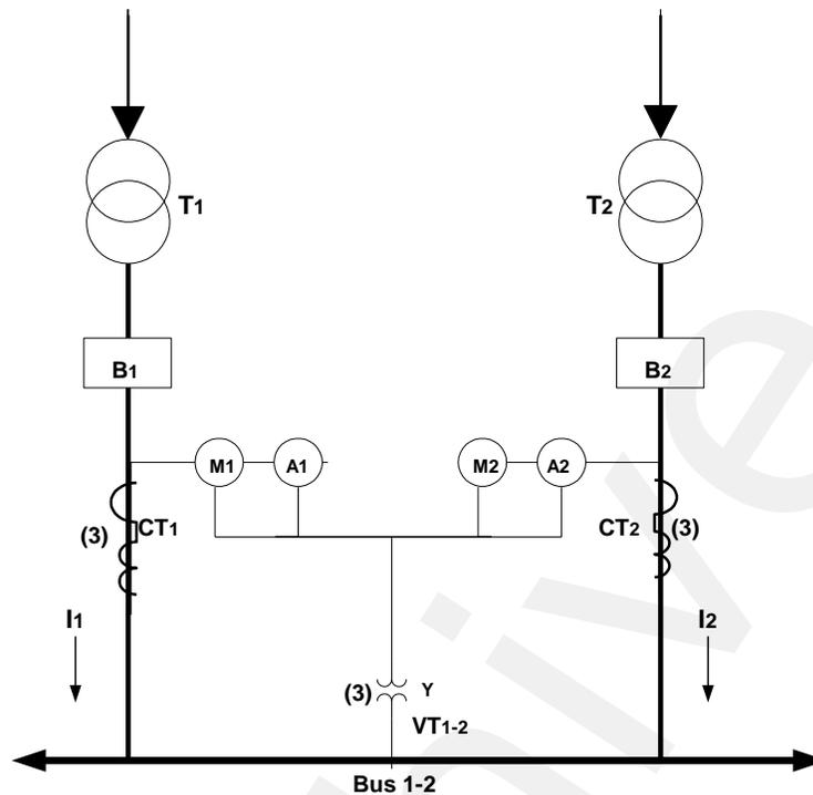
**Figure D-2: Six CTs and Three VTs in a Metering Installation for Two Equally-Loaded, Equivalent Transformers T<sub>1</sub> and T<sub>2</sub>, Connected to a Common Load Bus**
