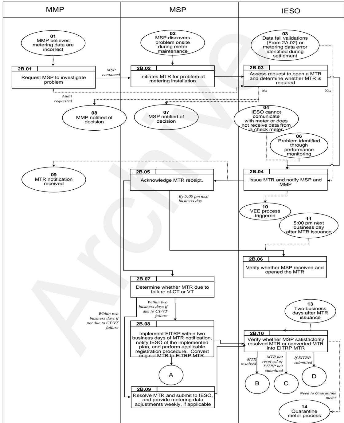
Figure 2–2: Work Flow for Meter Trouble Reports
