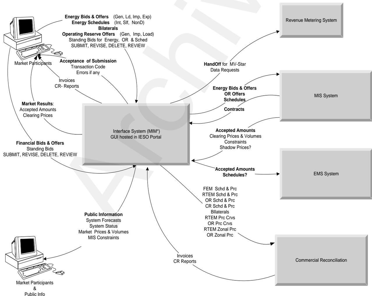
Figure 5-1: Overview of Dataflow from the MP to IESO systems
